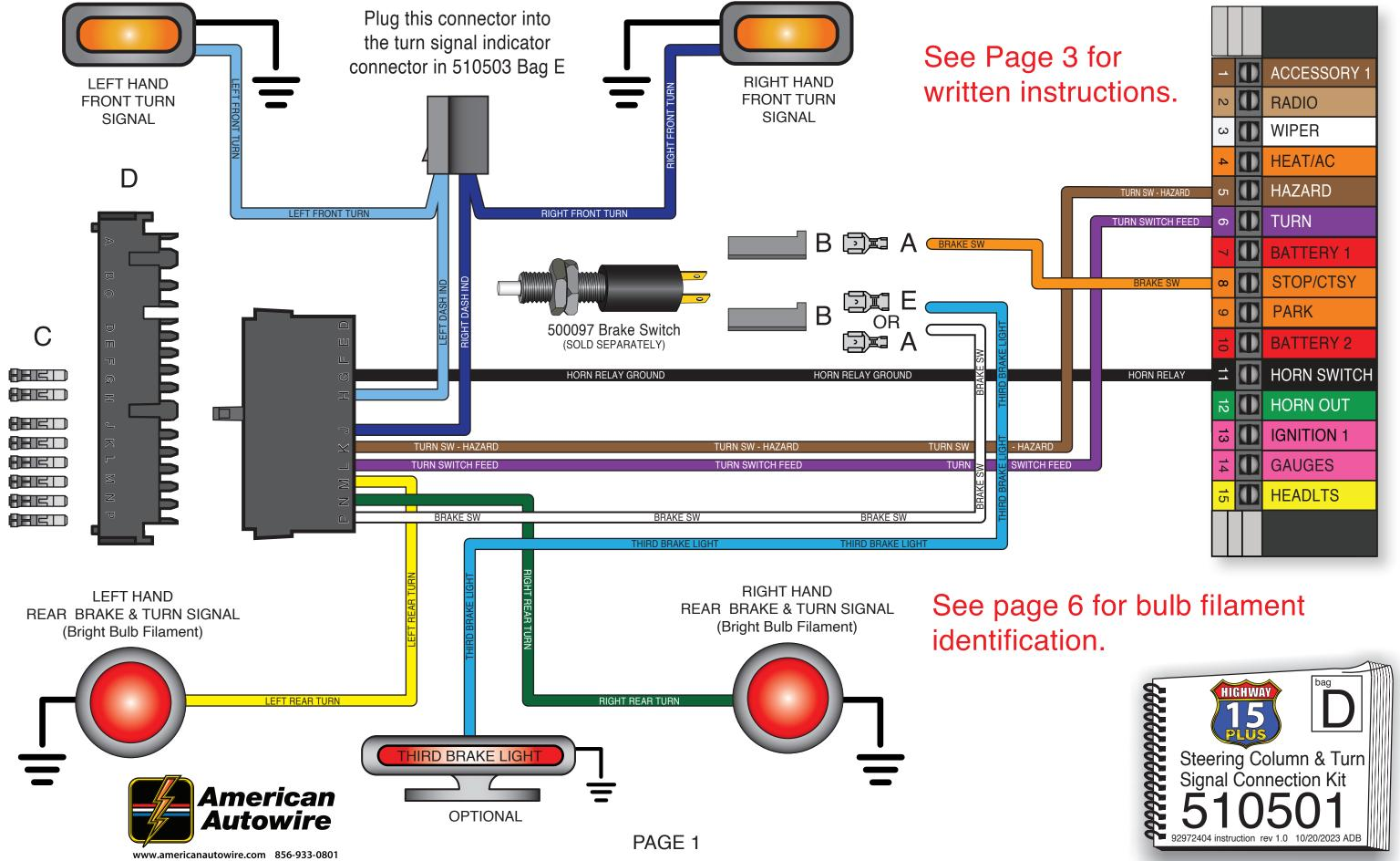
Use this diagram for vehicles with the brake & rear turn signals on separate bulbs:
